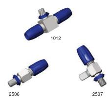
Omnifit variable bore adaptors allow any size of tubing between 0.5 and 4mm O.D. to be connected to a 1/4"-28 UNF port via the 'Omnifit Cap'. The valved version has a Tefzel® rotor. Each adaptor has a male 1/4"-28 UNF thread that will fit any female 1/4"-28 UNF threaded port.
