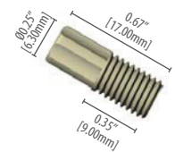
002145 Compact PEEK™ nut for 1/16" OD tubing, 1/4•28
